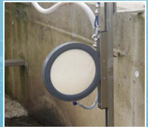
Figure 2: P700 Orthophosphate Analyzer 0.45 micron filter membrane on a slide rail
